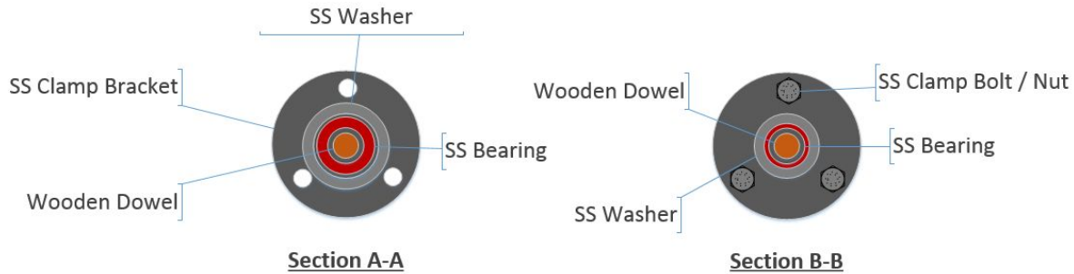
Figure 17: Control Gear / Servo motor Axis Construction
