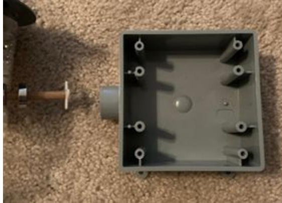
Figure 19: Electronics Housing Compartment
