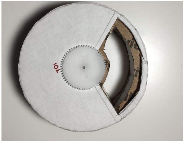
Figure 40: Bottom View of the Dispensing Disk
