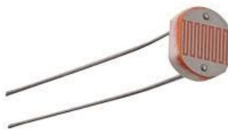
Figure 6 : Light Dependent Resistor (LDR) Sensor
