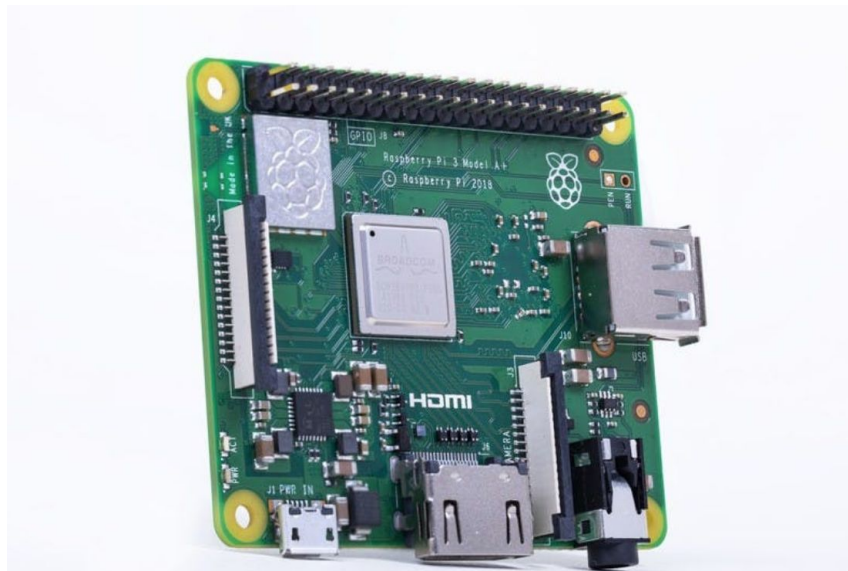
Figure 5: Raspberry Pi Model 3 A+
