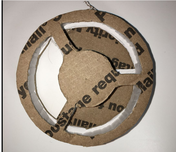
Figure 39: Top View of the Dispensing Disk
