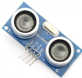
Figure 7 : HC-SR04 Ultrasonic Distance Sensor
